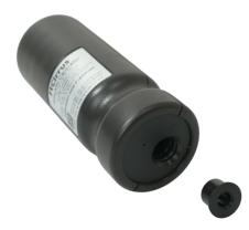
The battery-operated Class 1 Sound Calibrator 94 dB is classified for calibrating Class 1 measurement microphones, sound level meters, and other acoustic measurement equipment. This precision microphone calibrator delivers 94 dB at a frequency of 1 kHz.
